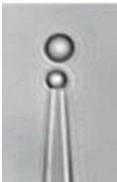
Figure 11. A: Video image of 2 \mu\text{m} bead on pipette with 3 \mu\text{m} bead above in trap. B: Recursive procedure “fillNeighbors” calls itself but returns when all interior pixels have been converted to dark (fillByte) level. Variables xSum and ySum divided by globSize give pixel-averaged x and y coordinates of bead.
