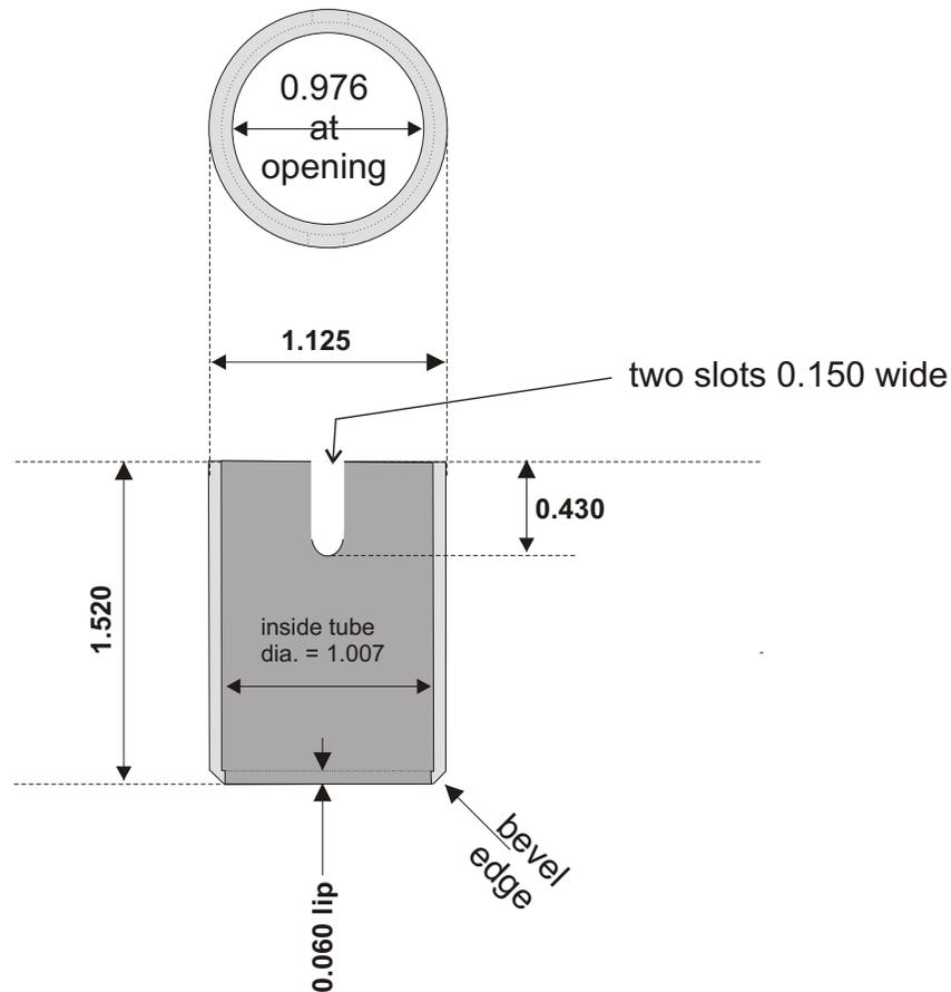
Note: Detector Holder Front will slide over Detector Holder Back with a smooth fit and the threaded holes will line up with the slots
